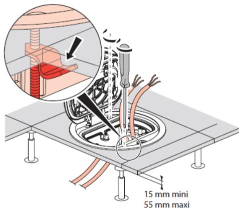
(4) Connect the mechanism with the cable. Don't forget the earth link
