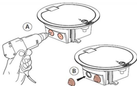
4) Place the cable in the cable protection
